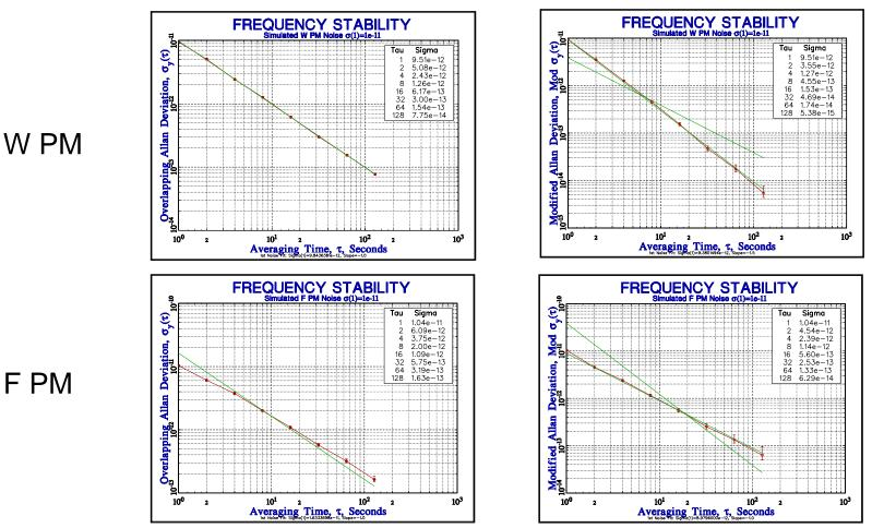
The W and F FM noise slopes are both  $\approx$  -1.0 on the ADEV plots, but they can be distinguished as -1.5 and -1.0 respectively on the MDEV plots.
