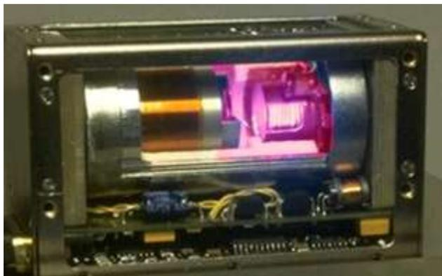
Figure 25. Photograph of Temex RFS with Cutaway Physics Package.
