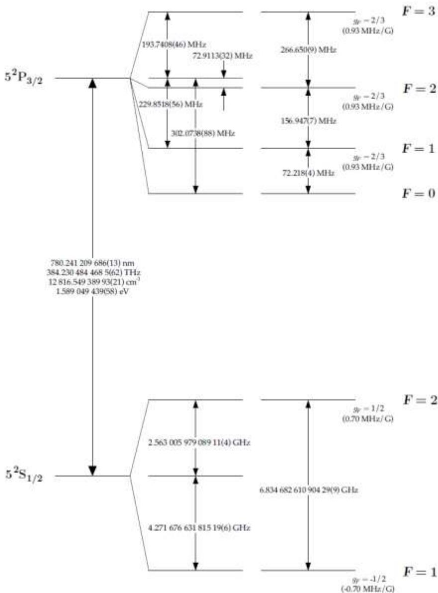
Figure 5.  $^{87}\text{Rb}$   $D_2$  Hyperfine Structure
