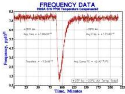
Figure 73. Temperature Compensated Transient Response
