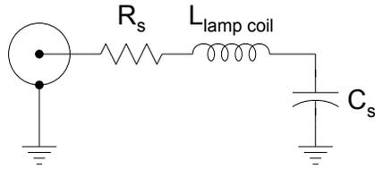
Figure 28. Lamp Test Circuit
