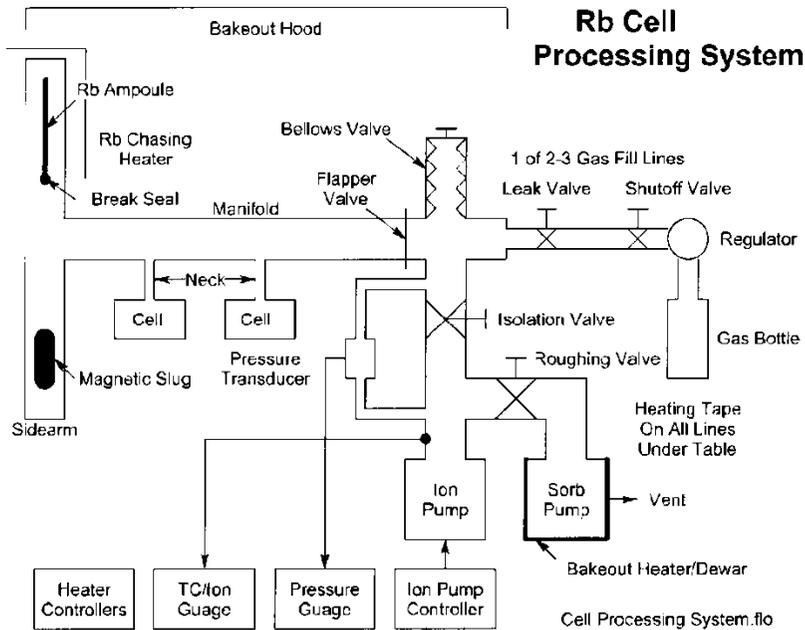
Figure 32. Typical Rb Cell Processing System
