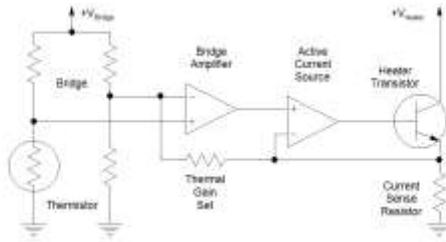
Figure 57. Basic Temperature Controller Circuit
