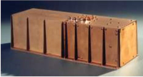
General Radio SATS (Spacecraft Atomic Timing System), c. 1970. First space qualified RFS. Rb frequency standard and digital clock.
