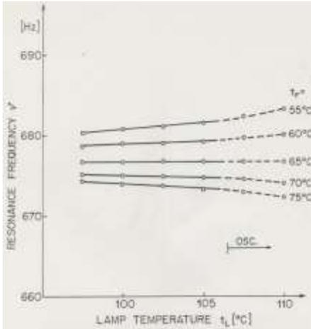
E. Frequency vs. Lamp Temperature
