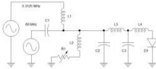
Figure 56. Typical SRD Multiplier Circuit
