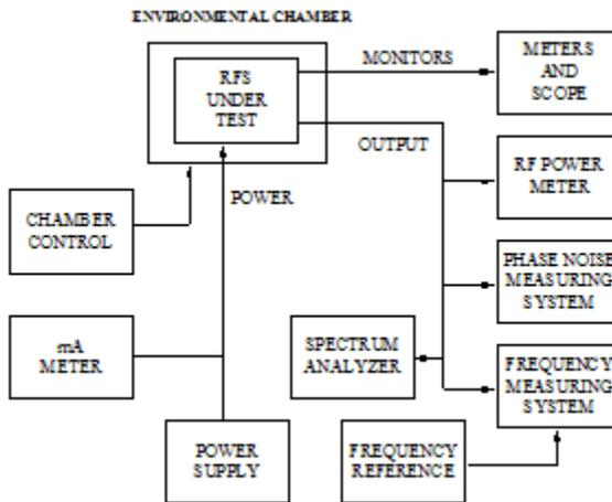
Figure 77. RFS Environmental Test Setup
