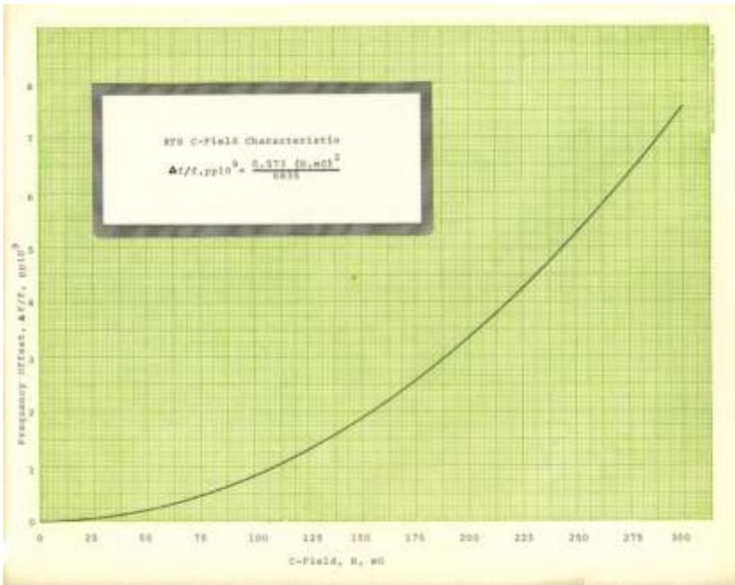
Figure 36. RFS C-Field Characteristic
