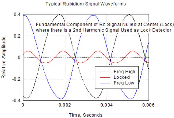
Figure 12. Rb Signal Waveforms
