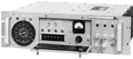
Collins Radio (later Rockwell Collins) AFS-81 Airborne RFS for Verdin VLF Communications system, c. 1970. Physics package built by General Radio. High performance, rugged.
