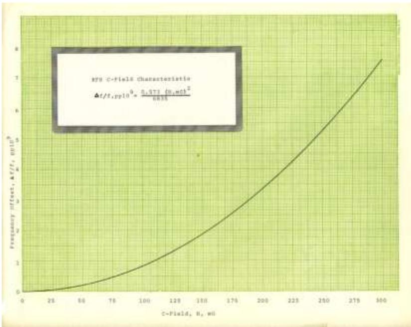
Figure 36. RFS C-Field Characteristic
