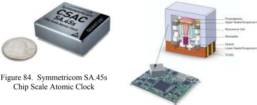
Figure 84. Symmetricom SA.45s
