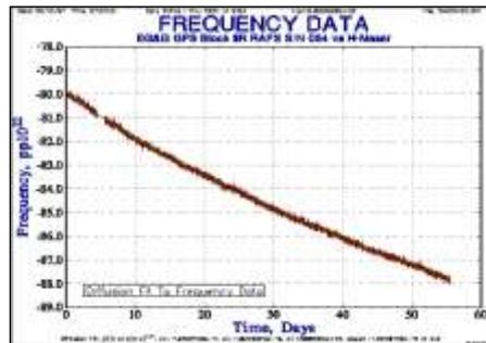
Figure 75. Diffusion Fit to RFS Aging
