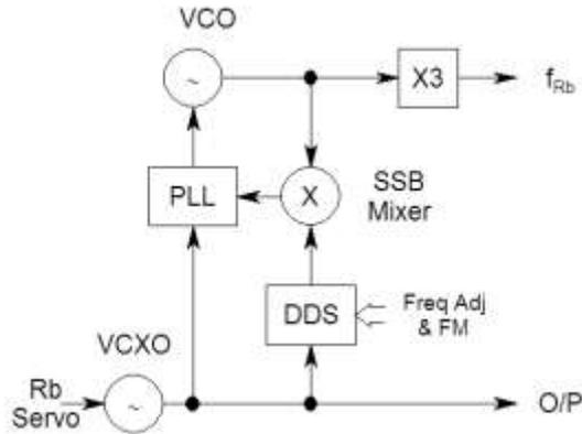
Figure 54. Modern Commercial RFS RF Chain
