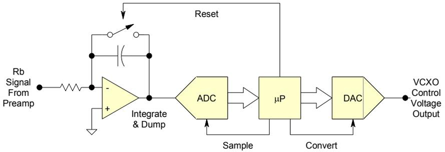
Figure 46. Integrate and Dump DSP Servo
