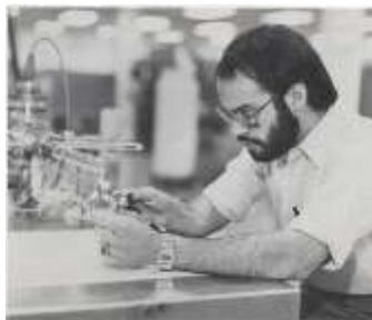
Figure 33. Pulling Lamps Off Vacuum System
