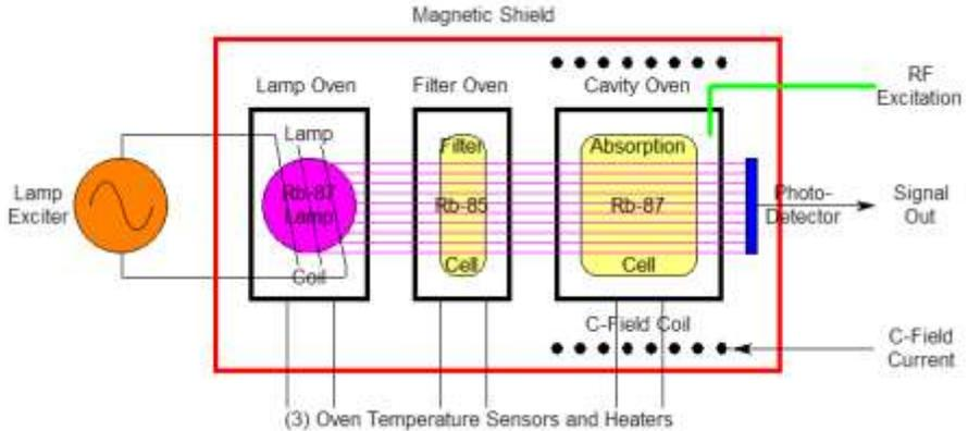
Figure 9. Schematic of a Classic RFS Physics Package
