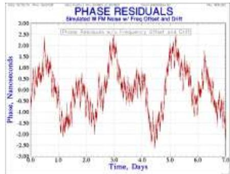
Figure 62. Phase Residuals without Frequency Offset Drift
