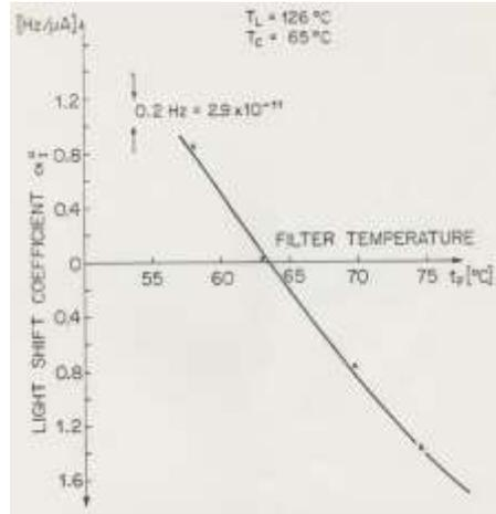
F. Light Shift Coefficient vs. Filter Temperature
