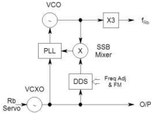
Figure 54. Modern Commercial RFS RF Chain
