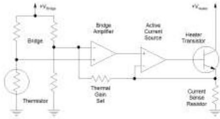
Figure 57. Basic Temperature Controller Circuit
