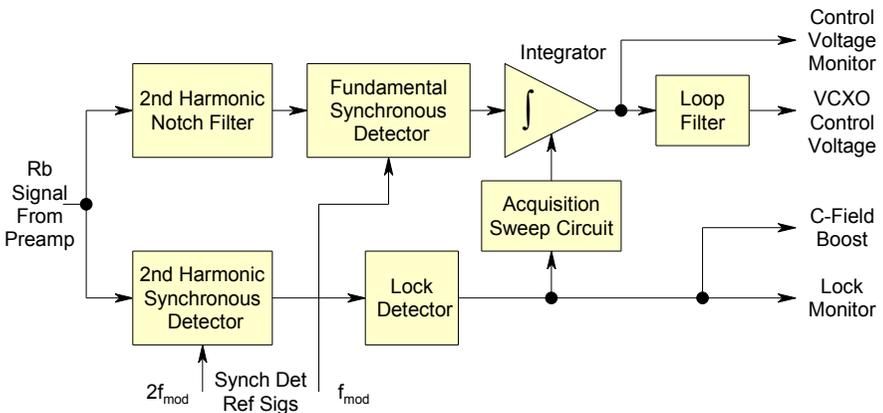
Figure 39. Typical Analog Servo Amplifier Block Diagram
