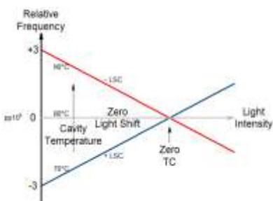
Figure 21. Characteristics of Tandem Cell RFS
