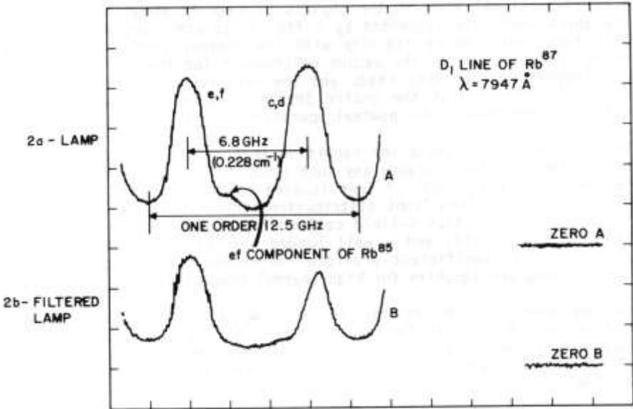
Figure 7. Unfiltered and Filtered Rb Lamp Spectrum
