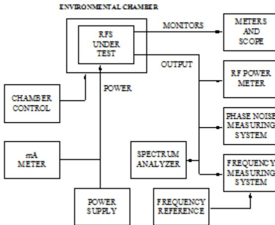
Figure 77. RFS Environmental Test Setup
