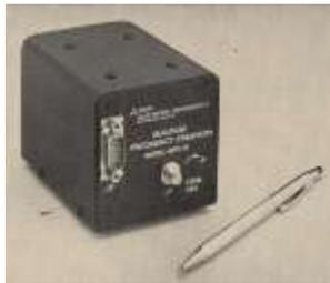
EG&G (later PerkinElmer and Excelitas) RFS-10 general purpose MIL RFS, c. 1985. Smaller version of M100 and RFS-10-7.
