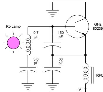
Figure 27. Basic Lamp Exciter Circuit
