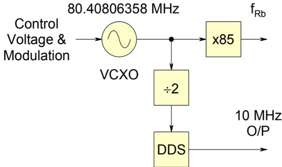
Figure 53 Simple Rb Clock RF Chain
