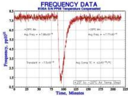
Figure 73. Temperature Compensated Transient Response
