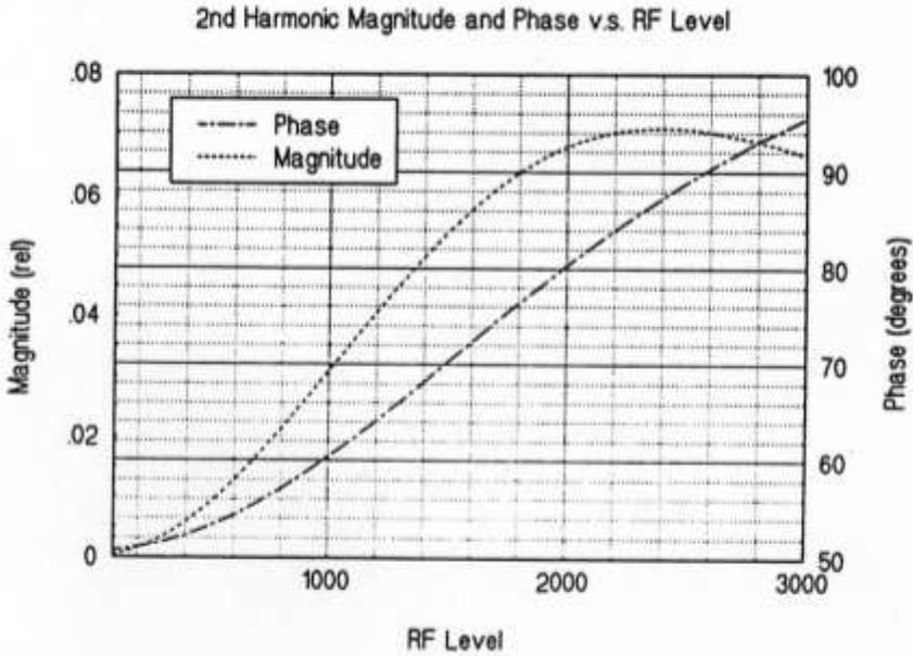
Figure 18. 2<sup>nd</sup> Harmonic Magnitude and Phase vs. RF Interrogation Power
