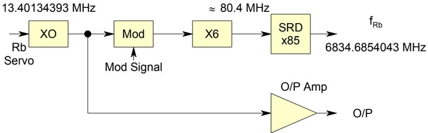
Figure 52. GPS RFS RF Chain
