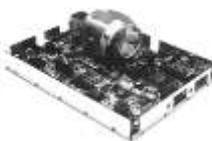
Efratom LPRO (Low Profile Rubidium Oscillator), c. 1995. Good performance, manufactured in large volumes for commercial telecom applications.
