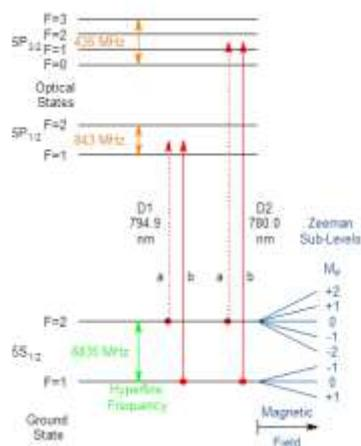
Figure 3. Energy Levels of  $^{87}\text{Rb}$
