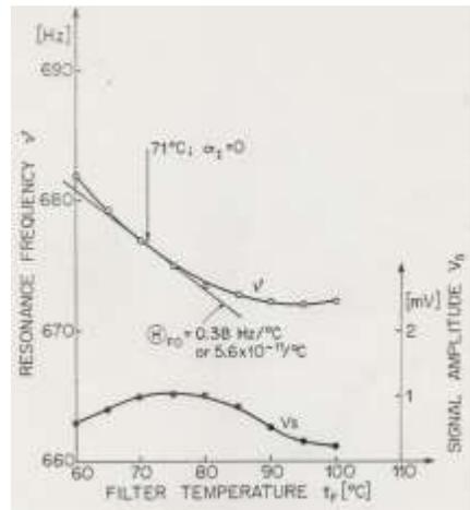
D. Frequency and Signal vs. Filter Temperature
