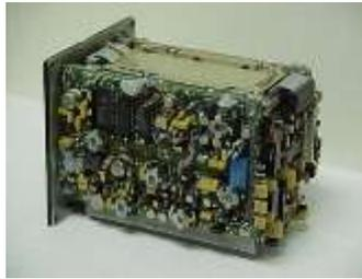
Efratom (later Ball Efratom) M3000 airborne tactical RFS, c. 1985. Similar units were built by EG&G and FEI. Probably the most environmentally hardened RFS units ever made.
