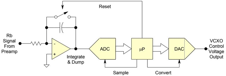
Figure 46. Integrate and Dump DSP Servo
