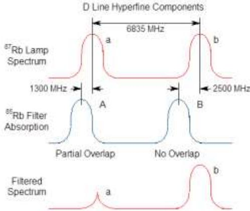
Figure 6. Isotopic Filtering of <sup>87</sup>Rb D Lines
