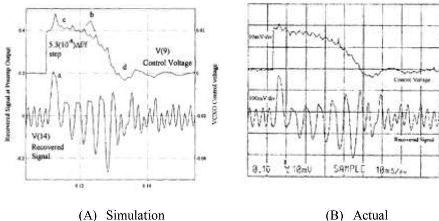
Figure 74. Servo Transient Response
