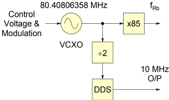
Figure 53 Simple Rb Clock RF Chain
