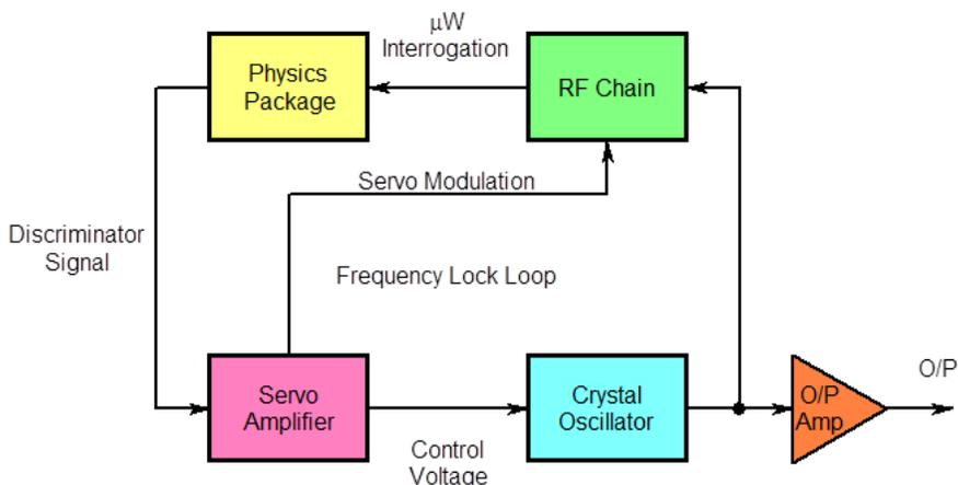
Figure 8. Block Diagram of a Passive Atomic Frequency Standard
