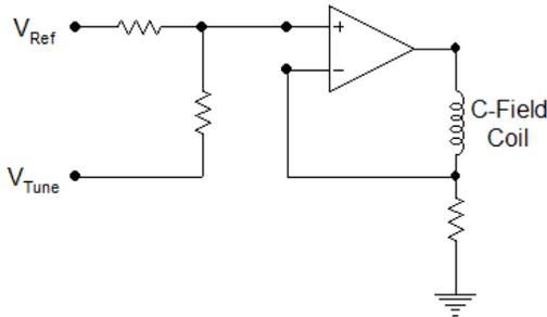
Figure 78. Typical C-Field Circuit
