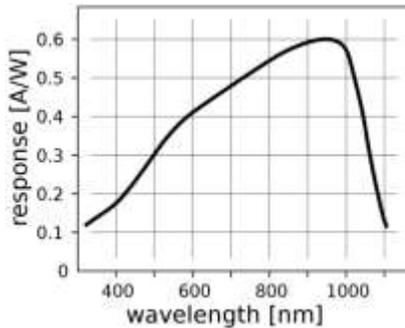
Figure 37. Si Photodiode Responsivity
