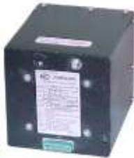
Efratom (later Ball Efratom, Datum and Symmetricom) M100 general purpose (e.g., ground anti-jam and troposcatter radio) MIL RFS, c. 1980. Similar RFS-10-7 made by EG&G.
