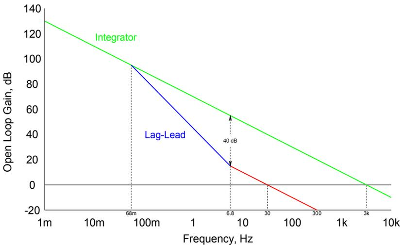
Figure 45. RAFS Servo Open Loop Gain (Log Approximation)
