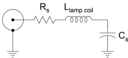
Figure 28. Lamp Test Circuit
