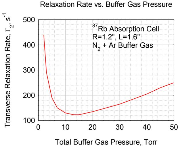
Figure 31. Linewidth versus Buffer Gas Pressure
