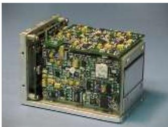
Symmetricom 8130A modern MIL-spec RFS, c. 2002. Re-placement for M100. Has DDS and digital control interface, screened PEMs.
