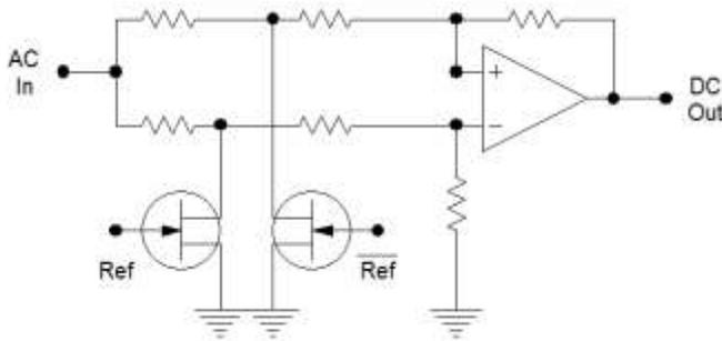
Figure 41. Basic Synchronous Detector Circuit
