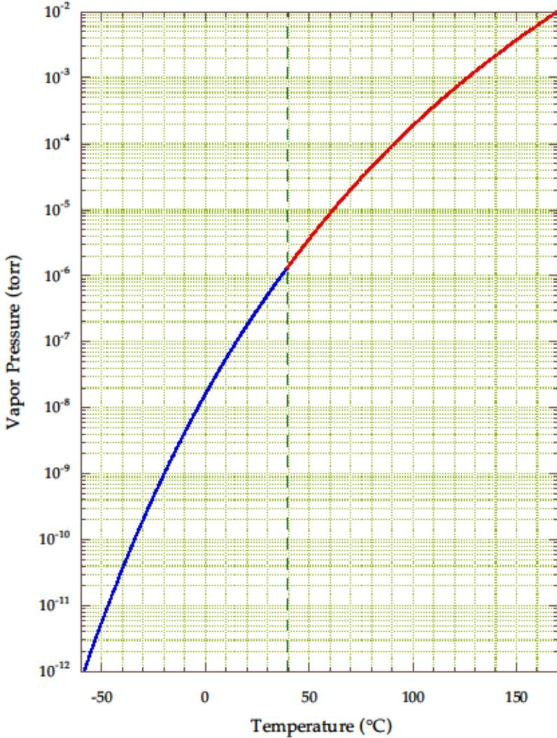
Figure 24. Rb Vapor Pressure vs. Temperature
