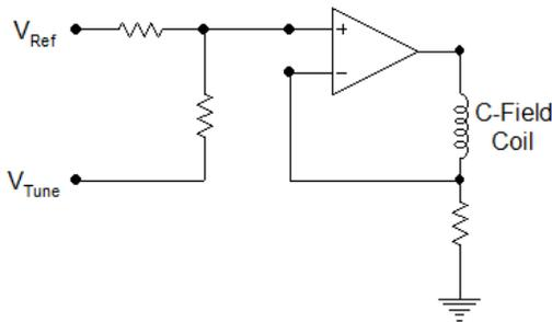
Figure 78. Typical C-Field Circuit
