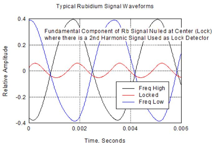
Figure 12. Rb Signal Waveforms
