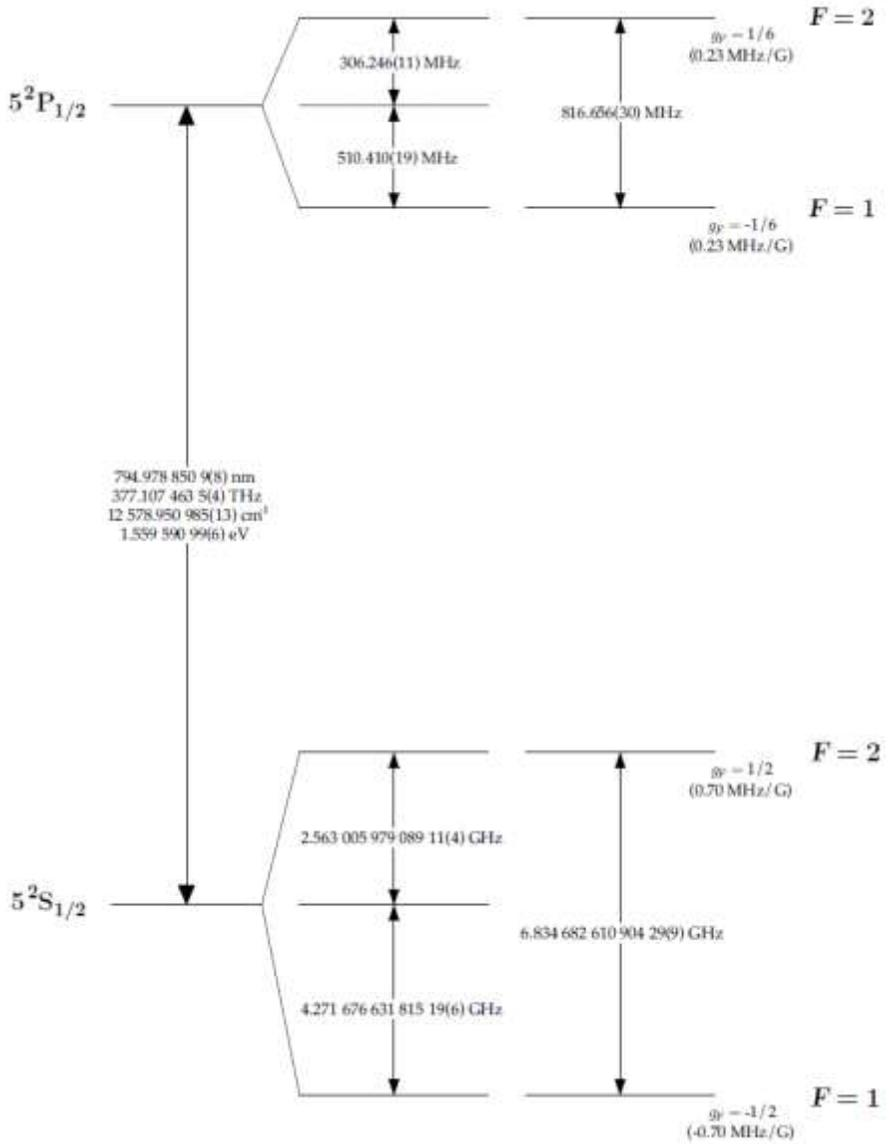
Figure 4.  $^{87}\text{Rb}$   $D_1$  Hyperfine Structure
