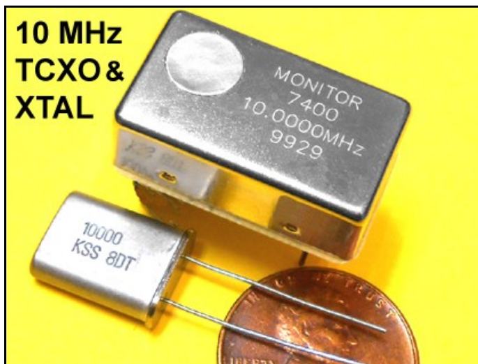
Figure 1. TCXO and Filter Crystal
