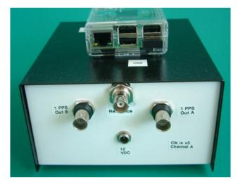
Figure 6. Rear Panel of TADD/TICC Enclosure
