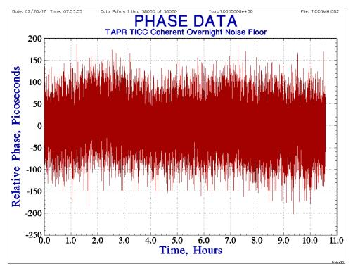
Figure 7. Phase Record for TADD-2/TICC Coherent Noise Test
