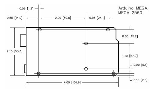
Figure 3. Arduino Mega 2560 Mounting Dimensions
