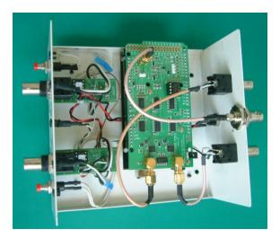
Figure 5. Interior of TADD/TICC Assembly
