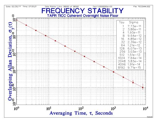
Figure 8. Stability Plot for TADD-2/TICC Coherent Noise Test
