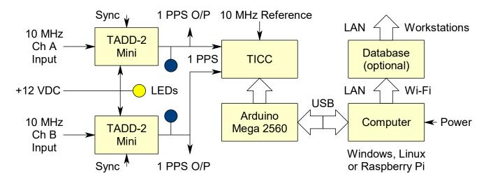
Figure 4. TADD/TICC System Block Diagram
