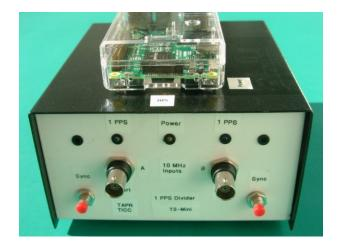
Figure 1. TADD/TICC Time Interval Counter (Shown with optional Raspberry Pi Computer)
