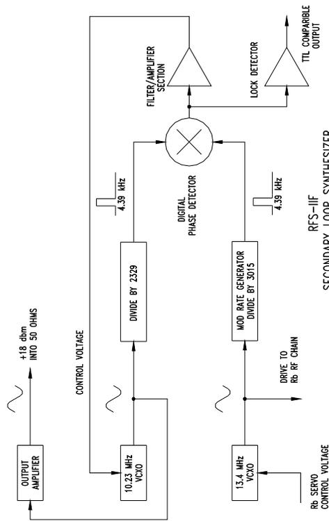
Figure 3. Synthesizer Block Diagram
